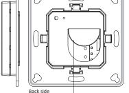
Battery: CR2430 Before the first use, please open the battery cover and remove the protective film.
